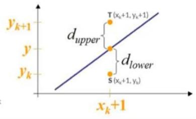
The recursive calculation of decision parameters is performed at each integer  $\mathbf{x}$  position, starting at the left coordinate endpoint of the line.
